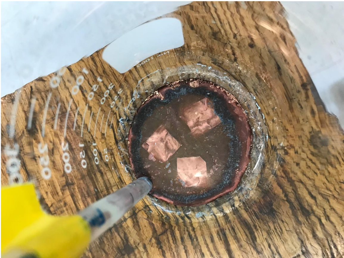
Figure 14: Experimental beaker after a foil test with a nitric acid, abrasion, and no pretreatment foil test. Note the prominent shadows left on the cathode where the foil was.
